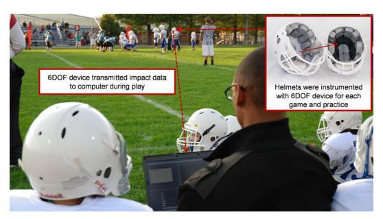
FIGURE 1. The helmets of youth football players were instrumented with the 6DOF head acceleration measurement device. Players wore instrumented helmets for every game and practice they participated in. Each time an instrumented player experienced a head impact, data were collected and then wirelessly transmitted to a computer on the sideline.
